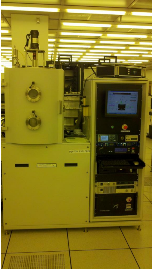
Denton Explorer – E-beam evaporator – metal deposition
