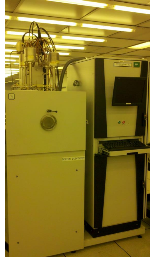
Denton Discovery – RF/DC sputterer – metal, dielectric
