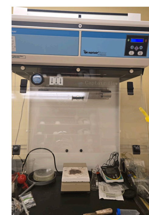
*Fume hood used for safe evaporation of chloroform
