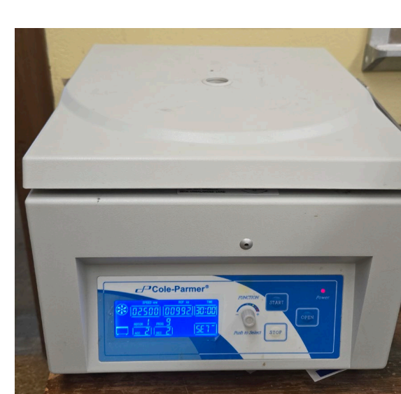
*Centrifuge used to separate mixture into layers
